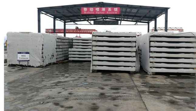
轨枕自动喷淋系统，减少水资源浪费 Automatic spraying system installed on sleepers to reduce the waste of water
